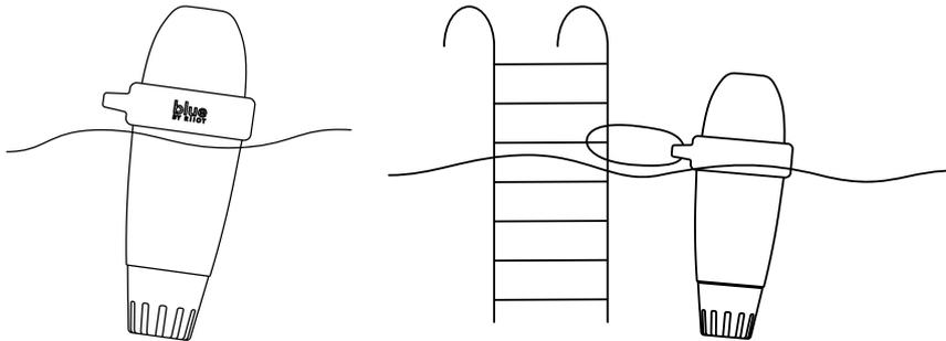
**NB:** Ensure that the **blue** floats vertically and that the head is clear of the water to allow correct communications with the device.
