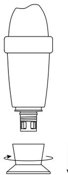
5. Empty the storage cap and rinse in clean water before returning it to the case.
